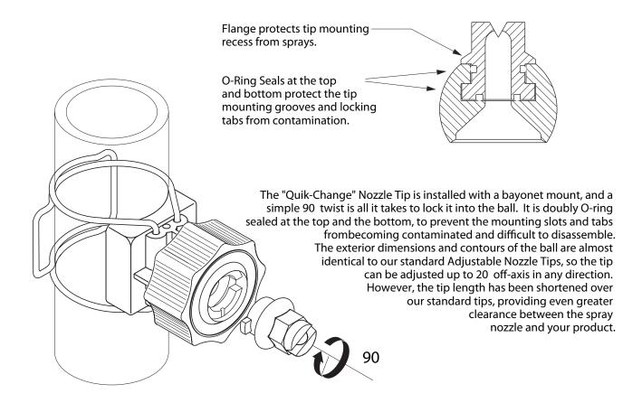
The Uni-Spray Systems "Quik-Change" Tip has been developed to meet our customers' demands! Manufactured to exacting standards from the highest quality engineered thermoplastics, the Quik-Change Tip demonstrates our on-going commitment to research and develop cost-effective, high performance replacement parts and innovative new products for the pre-treatment industry worldwide.
