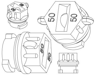
For easy identification, all flat Spray nozzle tips have the tip numbers molded into the ends of the tips. When ordering Nozzle Tips as spare parts, add 'TIP' after the part Number: e.g. 'UNI6540TIP'
